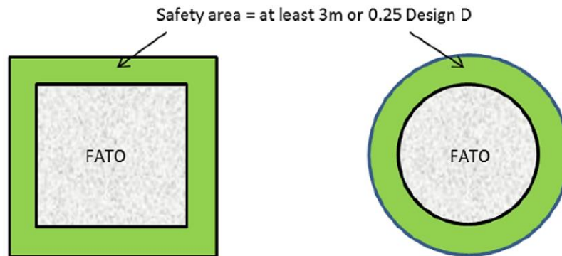
Figure 3-1: FATO and Associated Safety Area
